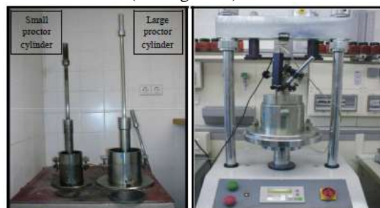
Fig. (2.11) Standard proctor instruments. Fig. (2.12) Computerized CBR-instrument, CBR-test conducted on tertiary clay specimen.
