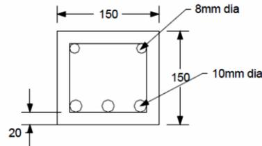
Figure 5.6 Cross Sectional Details of Flexure and Shear Beams (Size: 150mm x 150mm)
