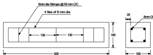
Figure 5.1 Reinforcement Details of Flexure Beams (Size: 100mm × 100 mm)
