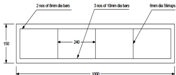
**Figure 5.5 Reinforcement Details of Shear Beams (Size: 150mm x 150mm)**
