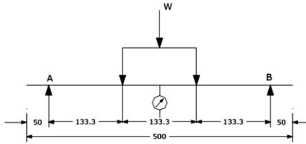
**Figure 5.19 Experimental Set up of Beam of Length 500 mm**
