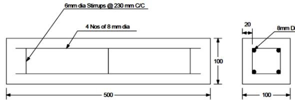
**Figure 5.2 Reinforcement Details of Shear Beams (Size: 100mm x 100 mm)**
