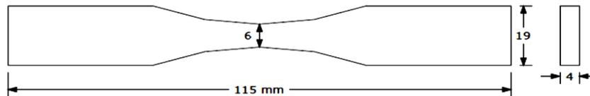
**Figure 5.3 FRP Tensile Test Specimen**
