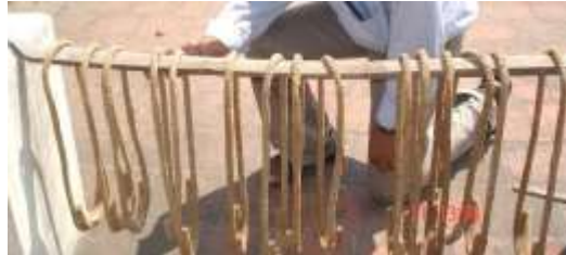
Figure 3.10 Curing of sand coated GFRP stirrups
