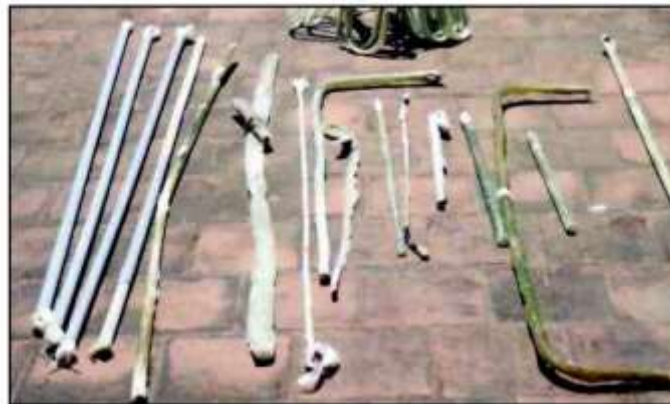
Figure 3.2 Some trail GFRP reinforcement specimens fabricated
