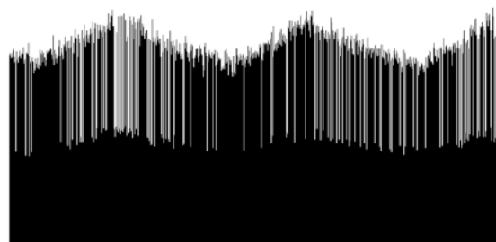
Figure 5.2: Overall ping power levels. The horizontal axis denotes the collection pings and the vertical axis denotes the average intensity of every ping [3]
