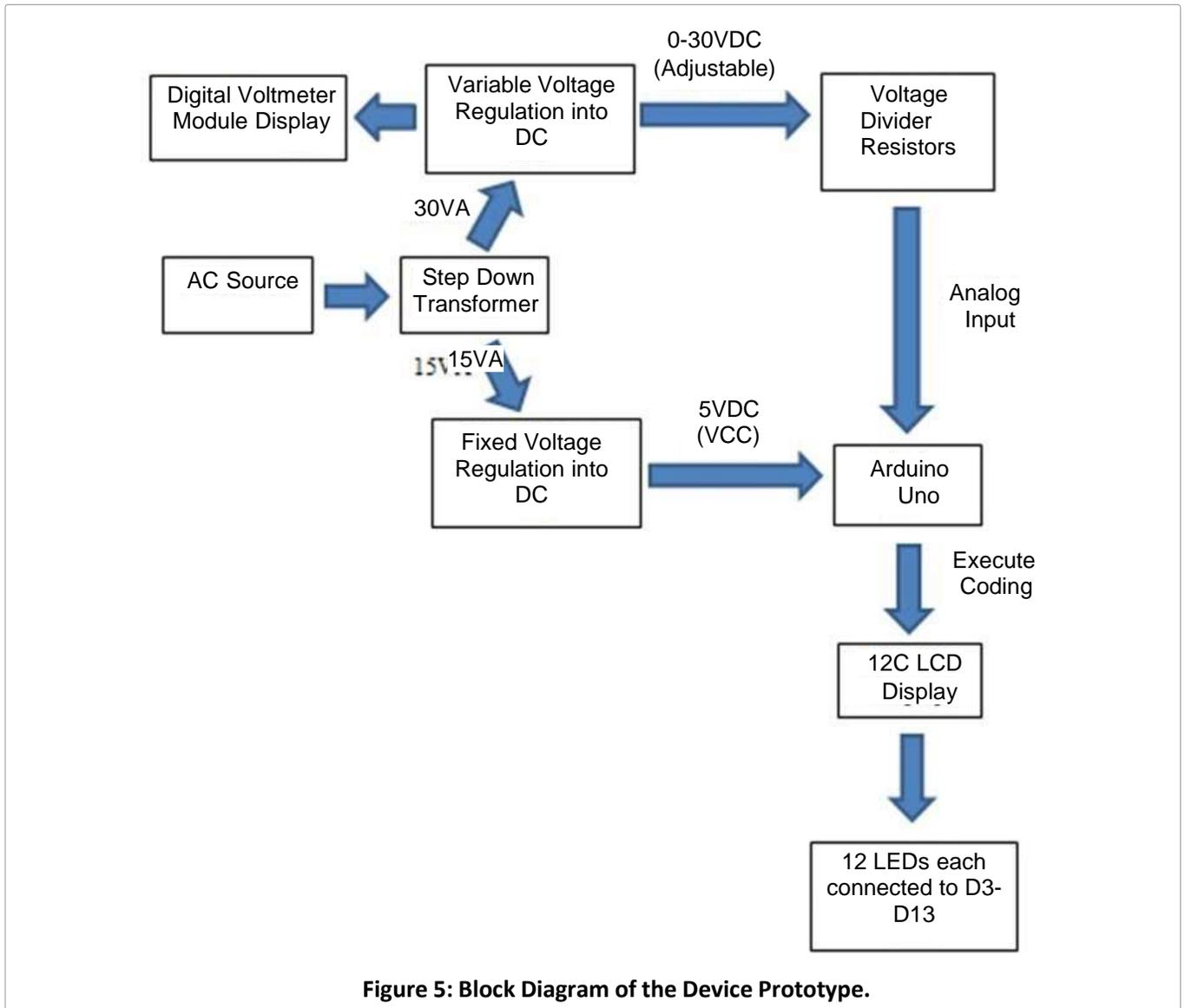
Figure 5: Block Diagram of the Device Prototype.
