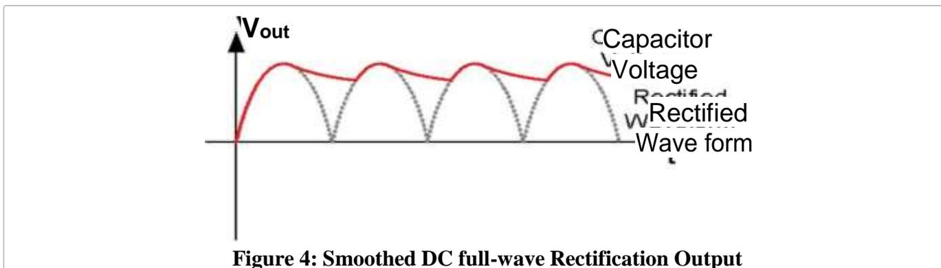
**Figure 4: Smoothed DC full-wave Rectification Output**
