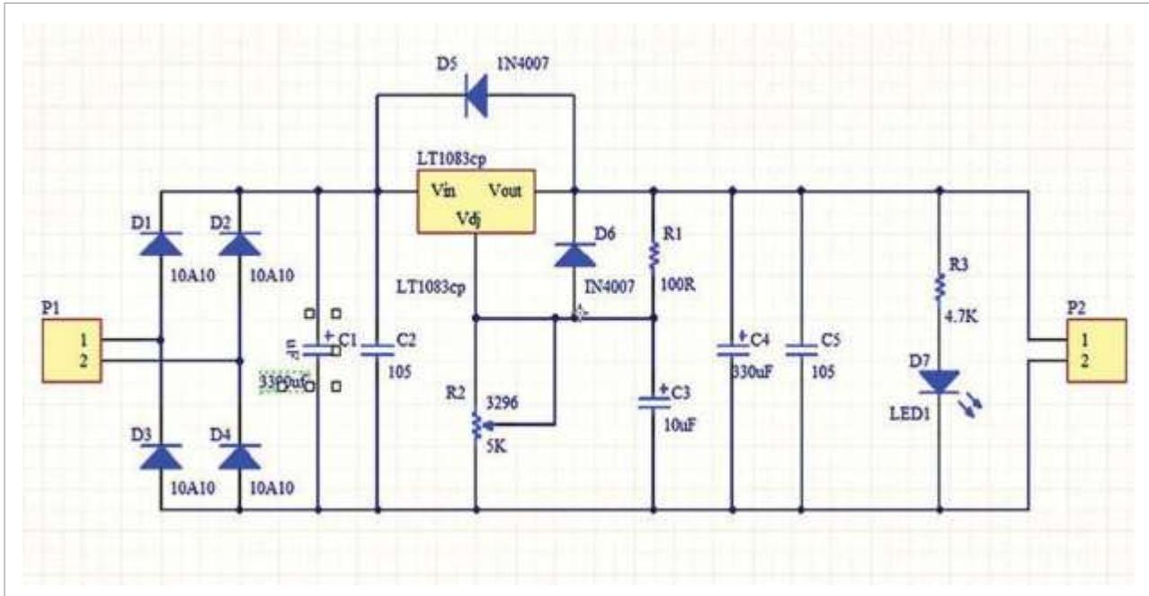
**Figure 4: Full Schematic of Variable Voltage Regulator.**
