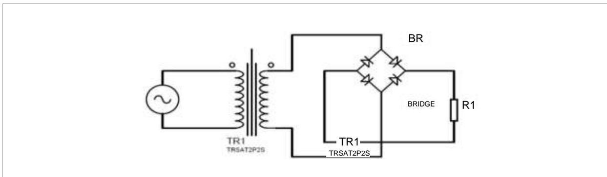
**Figure 3: Typical full-wave diode bridge Rectifier Configuration.**
