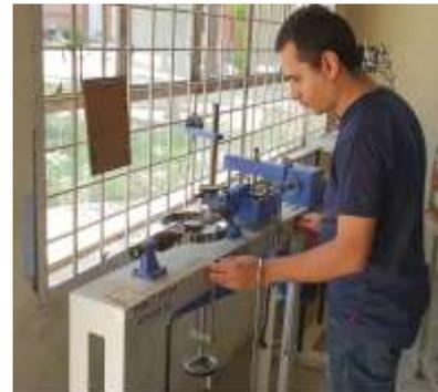
F 43.5 Experimental setup for direct shear test
