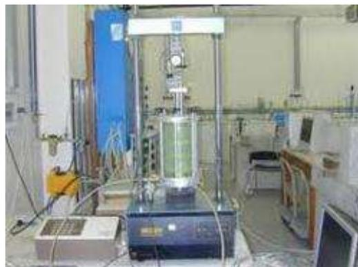
Fig. 3.6 Experimental setup for triaxial compression test
