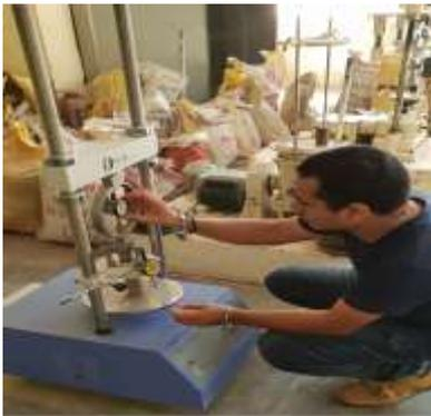
Figure 3.4 Experimental setup for unconfined compression test
