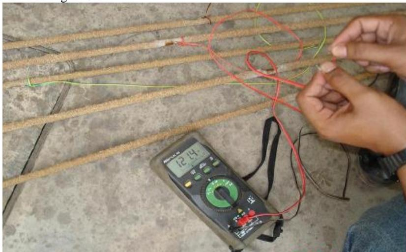
**Figure 3.11 Checking of strain gauges fixed over the GFRP bars**
