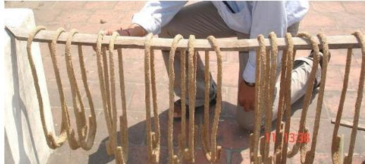
**Figure 3.10 Curing of sand coated GFRP stirrups**
