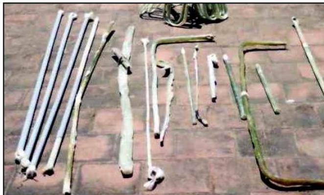
**Figure 3.2 Some trail GFRP reinforcement specimens fabricated**
