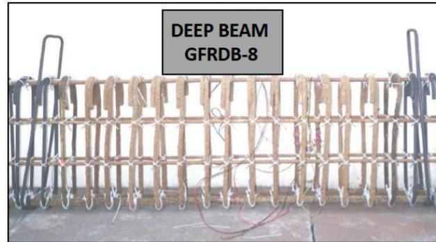
**Figure 3.12 Binding of GFRP reinforcement for beam GFRDB-8**
